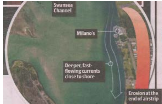
Restaurant Milano in Lake Macquarie collapsed due to soil erosion problems.
